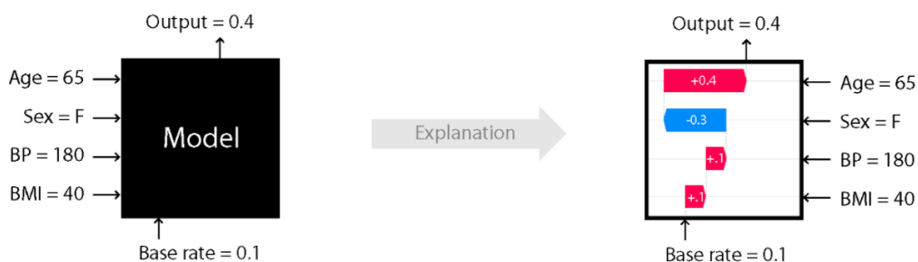
Figure 2.2.2 - A visualization of how SHAP works for a generic black-box model. The left-hand side shows Age, Sex, BP, BMI as input features and the output is an arbitrary prediction (0.4). The right-hand side shows the SHAP values colour-coded in terms of how much a feature contributes negatively (blue) or positively (red) for the given prediction. The SHAP values can be interpreted as the impact of having a certain value for a given feature in comparison to the same prediction if that feature had a baseline value.
